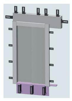
using the pull-down menu (in 100 mm steps) or freely entered by hand. Door frame dimensions, such as FW (frame width), FD (frame depth), and FH (frame height) can be freely entered within a defined range; users are however always first referred to the most favourable standard dimensions. Various types of electrical protection can be configured, as can numerous door panel constructions. A control panel section can be optionally displayed in
