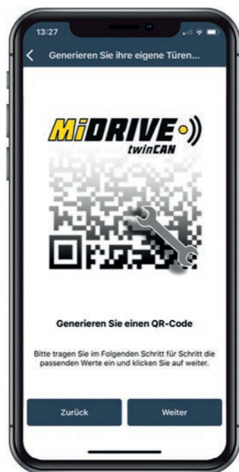
The commissioning of MiDrive has been enhanced by a wizard. This allows the most common configurations to be easily set for optimum door travel.
