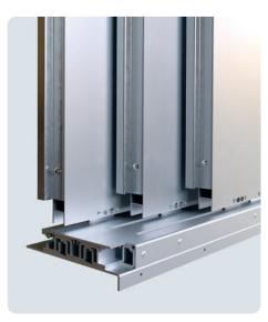
The high load bearing steel sill is always in two parts. The guide grooves are lasered only as far as this is necessary for the travel of the door panels. This means that guide grooves are not visible when the door panels are closed. The sill's maximum wheel load is 5.0 t.
