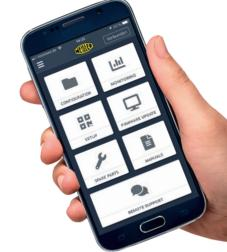
It involves the use of predefined QR codes to configure the door on site, in accordance with the product and order. In addition, special QR codes allow service technicians to respond quickly and easily in the event of any problems. Error codes are displayed in clear text form on the smartphone screen, enabling uncomplicated fault analysis at any time.
